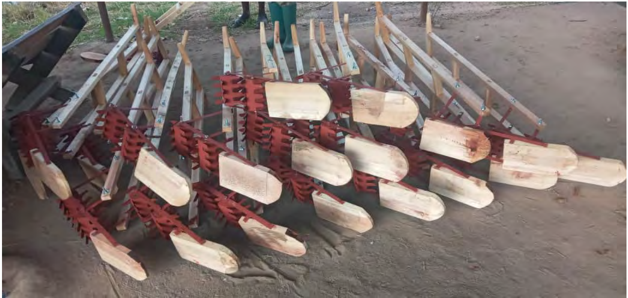
Locally made push weeder for rice for distribution to farmers
